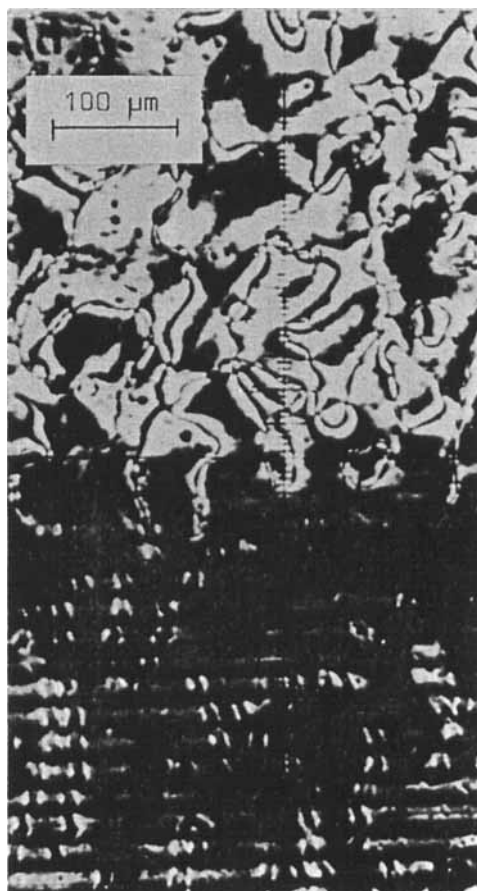
Figure 3. Micrograph of a LC layer between crossed polarizers. The supporting glass plates were partly scratched. Width of scratches: 1 \mu\text{m} ; spacing of scratches: 25 \mu\text{m} .
